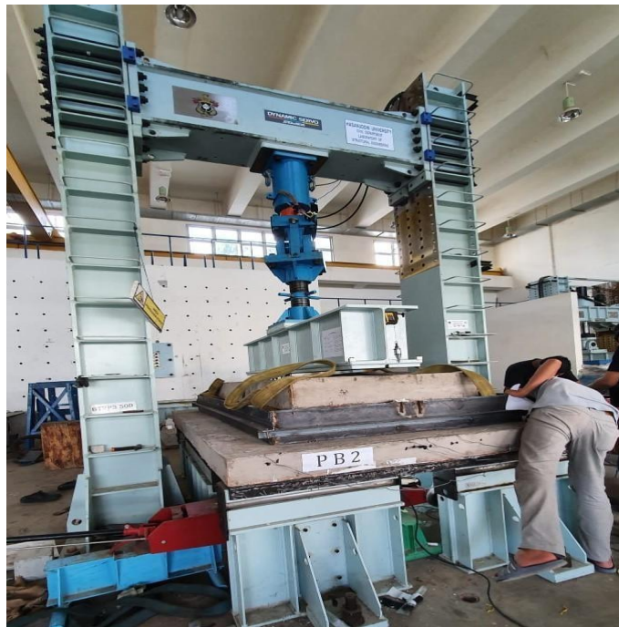
Figure 10. Hollow Plate Loading Pattern (PB-2)
