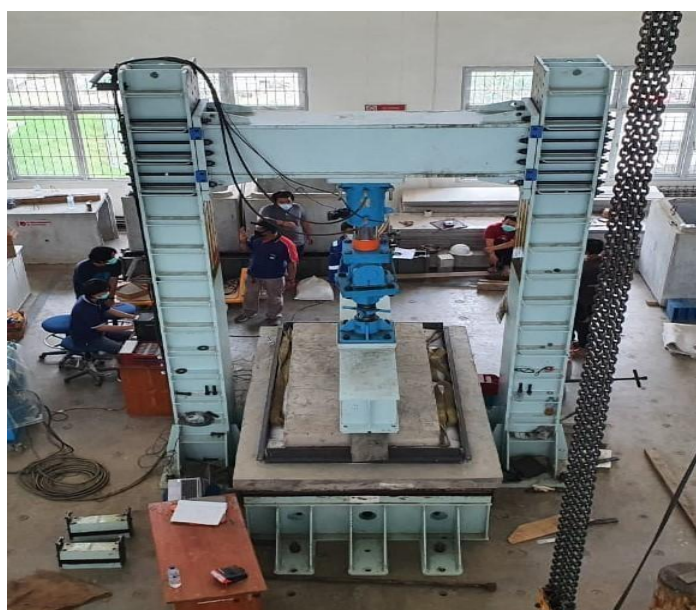
Figure 9. Solid Plate Loading Pattern (PP-1)
